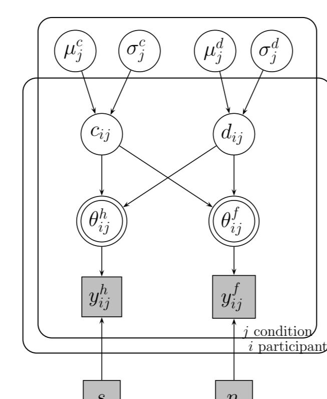
$$\begin{aligned} \mu_j^d &\sim \text{Gaussian}(0, 1)_{T(0,6)} \\ \mu_j^c &\sim \text{Gaussian}(0, 0.7) \\ \sigma_j^c, \sigma_j^d &\sim \text{Uniform}(0, 4) \\ d_{ij} &\sim \text{Gaussian}(\mu_j^d, \sigma_j^d) \\ c_{ij} &\sim \text{Gaussian}(\mu_j^c, \sigma_j^c) \\ \theta_{ij}^h &= \phi(\frac{1}{2}d_{ij} - c_{ij}) \\ \theta_{ij}^f &= \phi(-\frac{1}{2}d_{ij} - c_{ij}) \\ y_{ij}^h &\sim \text{Binomial}(\theta_{ij}^h, s) \\ y_{ij}^f &\sim \text{Binomial}(\theta_{ij}^f, n) \end{aligned}$$
